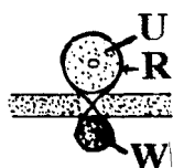
FIG. 1b—An enlarged cross section view of the AB wall with a hole through which the method of passing the rubber band holding the bone is shown. H = Holes, R = Rubber band, S = Slider, T = Thread, U = Ulna bone, and W = Wooden stay.
